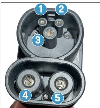
Fig. 17: Charge plug CCS Combo-2
