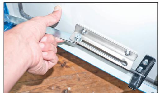
Fig. 18: releasing the locking rail
