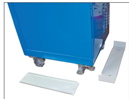
Fig. 41: removed base panels for ECC 320
