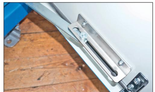
Fig. 19: released locking rail
